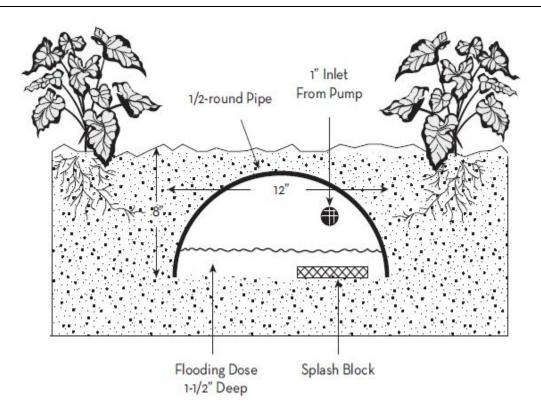
Figure D-5 Graywater Irrigation Chambers
