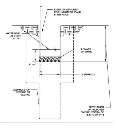
Figure B-1 Soil Percolation Test Arrangement
