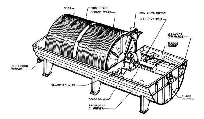
Figure F-4 Rotating Biological Contactor (RBC) Schematic
