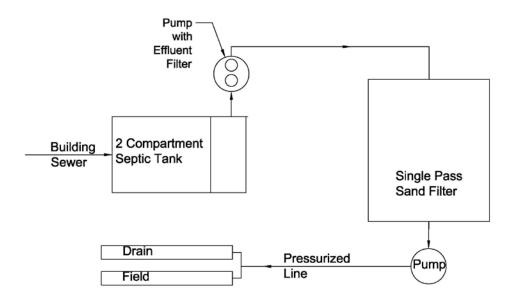
Single Pass Sand Filter and Pressurized Discharge to Drainfield
