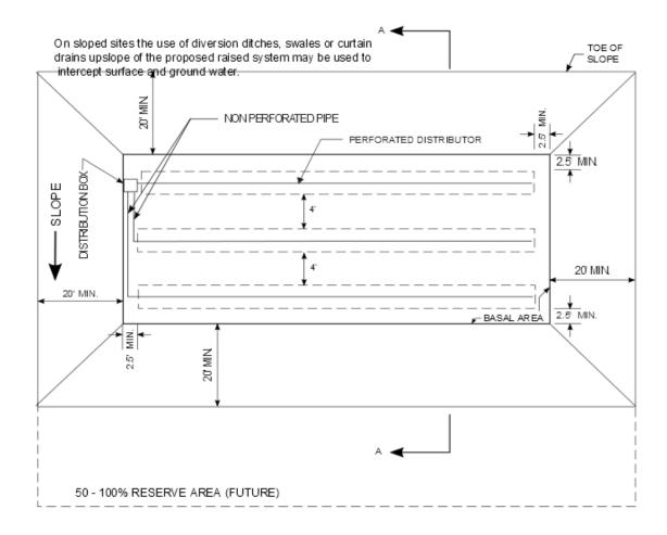
NOTE S: 1. There is at least one foot of original soil with faster than 60 minutes percolation rate, above any impermeable soil layer or bedrock, but not more than two feet.
