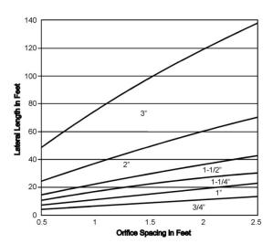
Figure A-2a: Minimum lateral diameter based based on orifice spacing for 3/16" diameter orifices
