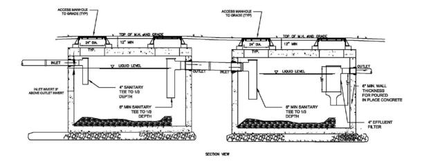
Figure D-4 Single-Compartment Septic Tanks in Series
