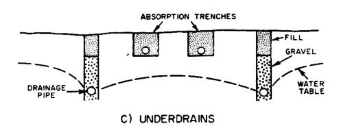
Figure E-13 Subsurface Drainage Methods
