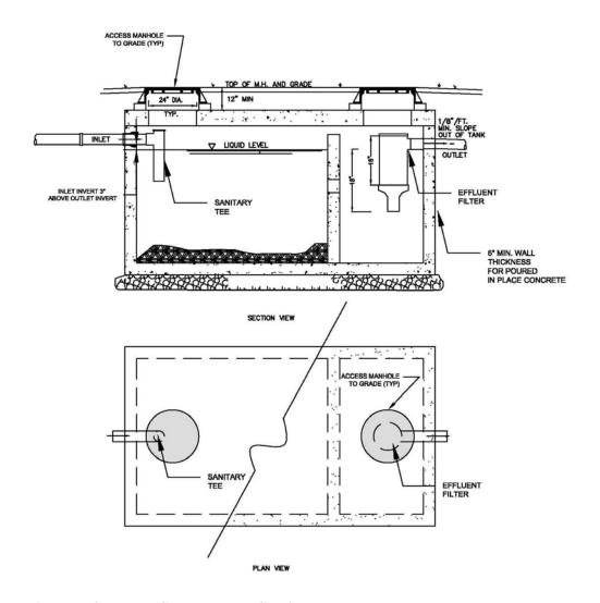
**Figure D-3 Double Compartment Septic Tank**
