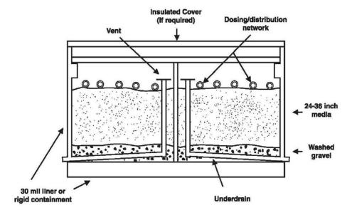
Figure F-2 Open Single-Pass Sand Filter
